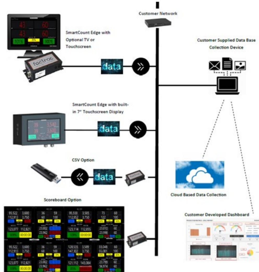
**Display** individual KPI data at the machine with a SmartCount Edge or SmartCount Edge-7
